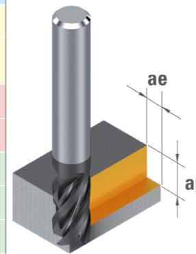
$$n [\text{rpm}] = \frac{V_c [\text{m/min}] \times 1000}{\pi \times D_1 [\text{mm}]}$$
