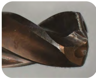
Significant wear after 60 holes
