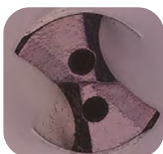
Holes \varnothing 0.15 Conventional drill
