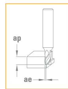
$$n [\text{tr/min}] = \frac{V_c [\text{m/min}] \times 1000}{\pi \times D_1 [\text{mm}]}$$
